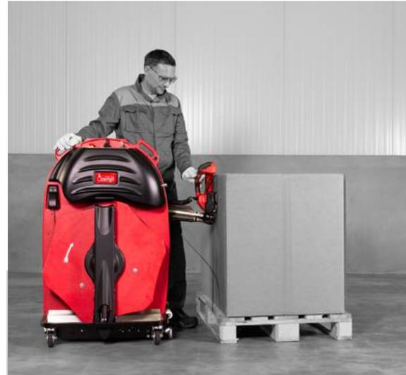
The strap lifter brings the 2nd strap end. The **sealing head** welds the strap securely.
