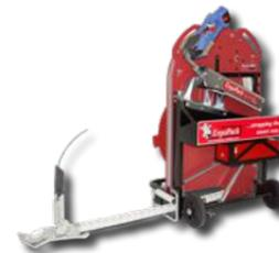
Change from the crank to an electronic drive operated by battery. The ErgoPack Tool-Lift makes side strapping of high pallets even easier, as different sealing tools can be attached to it and do not have to be held in the hand.
