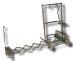
First prototype of a strapping device based on a double scissors system similar to a scissors lifting table.
